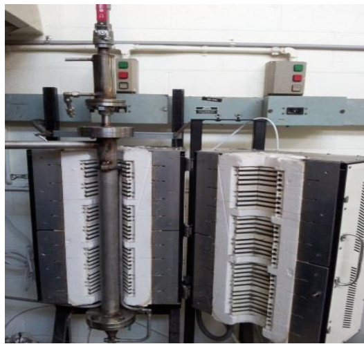
Figure 3-2 Bench scale fluidized bed reactor
