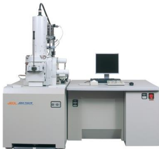
Figure 3-7 JOEL 7001F SEM with an Oxford Instruments X-Max 80 Silicon Drift EDS detector [7]
