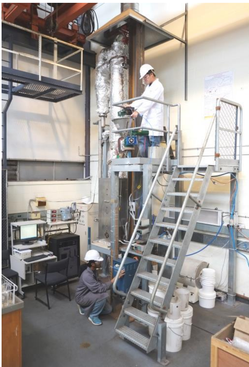
Figure 3-6 Photograph of the 10 kW th fluidized bed reactor
