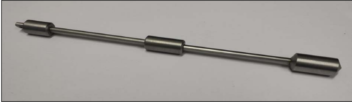
Figure 34 Custom-made Molybdenum Spindle and bob
