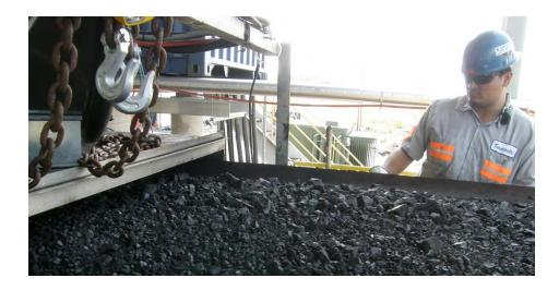
Figure 31: Microwave dried coal emerging from the drying zone (© Drycol Australia)
