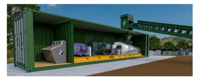
Figure 14: Artist's impression of the modular Ahrko swirling flow coal dryer (© Ahrko Systems)
