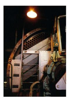
Figure 5: ZEMAG rotary tubular steam dryer at Morwell briquette factory (Allardice 2015)
