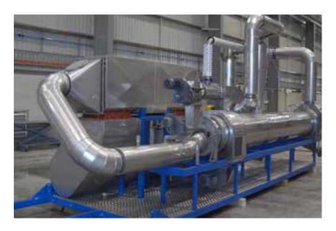
Figure 2: Pilot scale superheated steam rotary drum dryer (© Keith Engineering (Australia))
