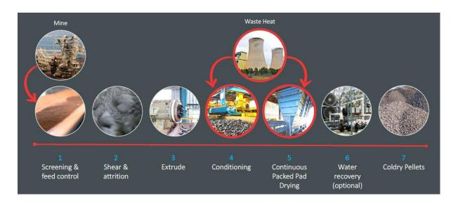
Figure 39: Overview of Coldry process (© ECT)
