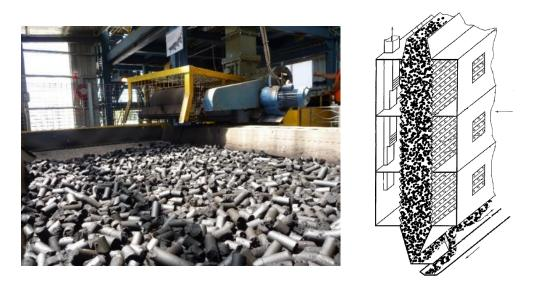
Figure 40: ECT's extruded densified brown coal pellets and dryer design (© ECT)
