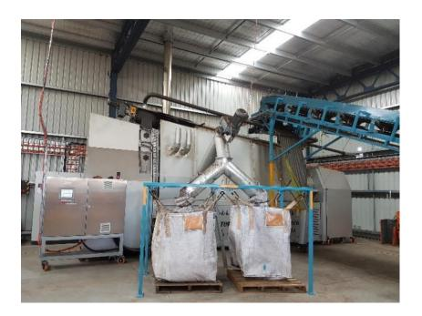
Figure 34: Pilot-scale torrefaction reactor (© Torreco)
