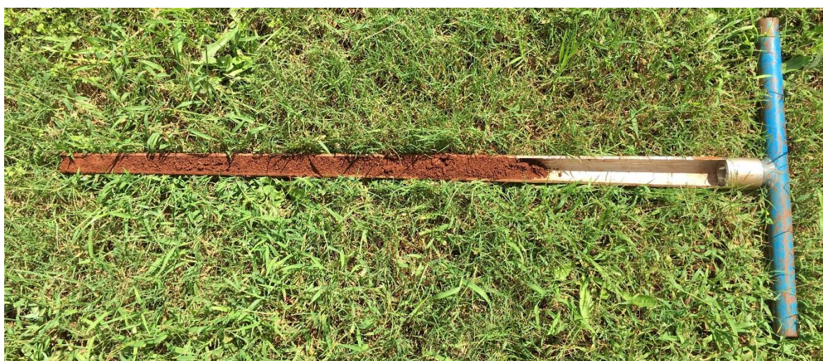
Figure 6.2. Collection of soil with hand auger
