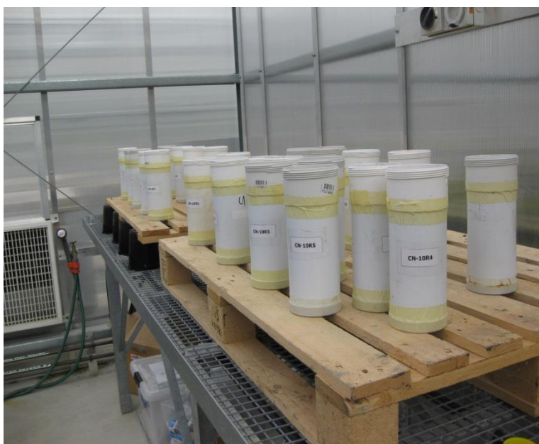
Figure 7.6. Incubation of soil in PVC tubes at 22\pm 1^{\circ}\text{C} in the glasshouse
