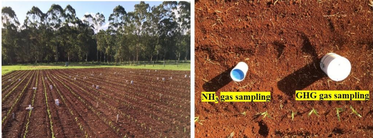
Figure 5.1. Experimental set up (left) and greenhouse gas (GHG) sampling (right) of sweet corn in the field
