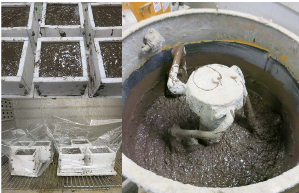
Figure 3.5 Loy Yang brown coal fly ash geopolymer concrete: mixing; moulding; and elevated temperature curing.
