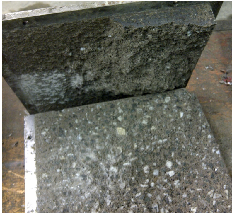
Figure 5.7 Broken specimen Loy Yang brown coal fly ash geopolymer concrete when demoulded
