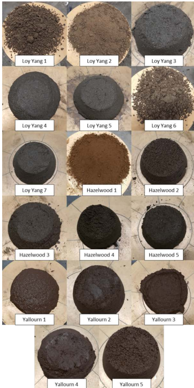
Figure 4.7 Image of Loy Yang, Hazelwood and Yallourn brown coal fly ash geopolymer mortar mixtures after flow table test
