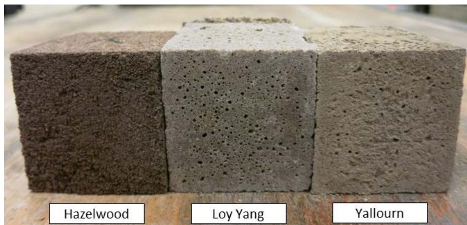
Figure 3.10 La Trobe Valley brown coal fly ash geopolymer mortar: Yallourn, Loy Yang and Hazelwood
