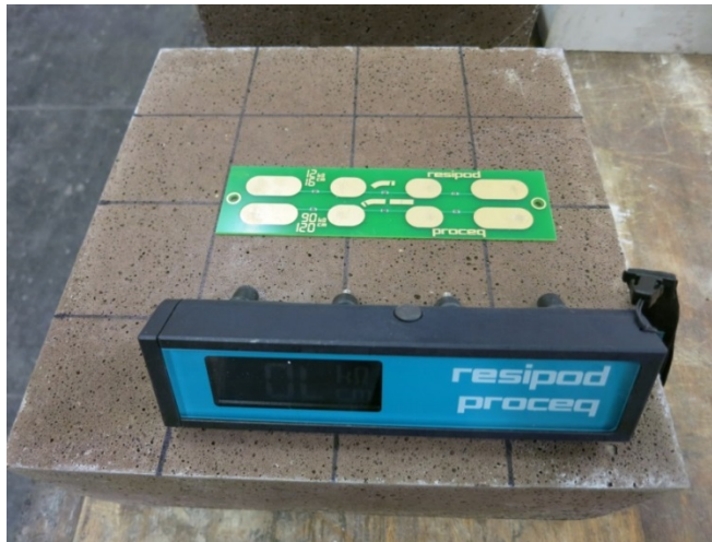
Figure 3.14 Electrical resistivity test equipment
