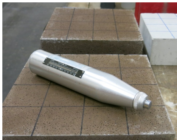
Figure 3.12 Schmidt Rebound Hammer equipment
