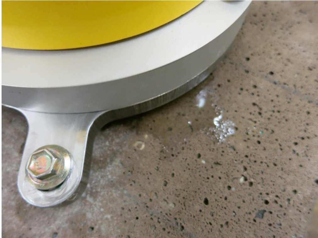
Figure 5.15 Surface pore water leaking during water absorption (sorptivity) test Loy Yang brown coal fly ash geopolymer concrete sample Batch 1-(i)
