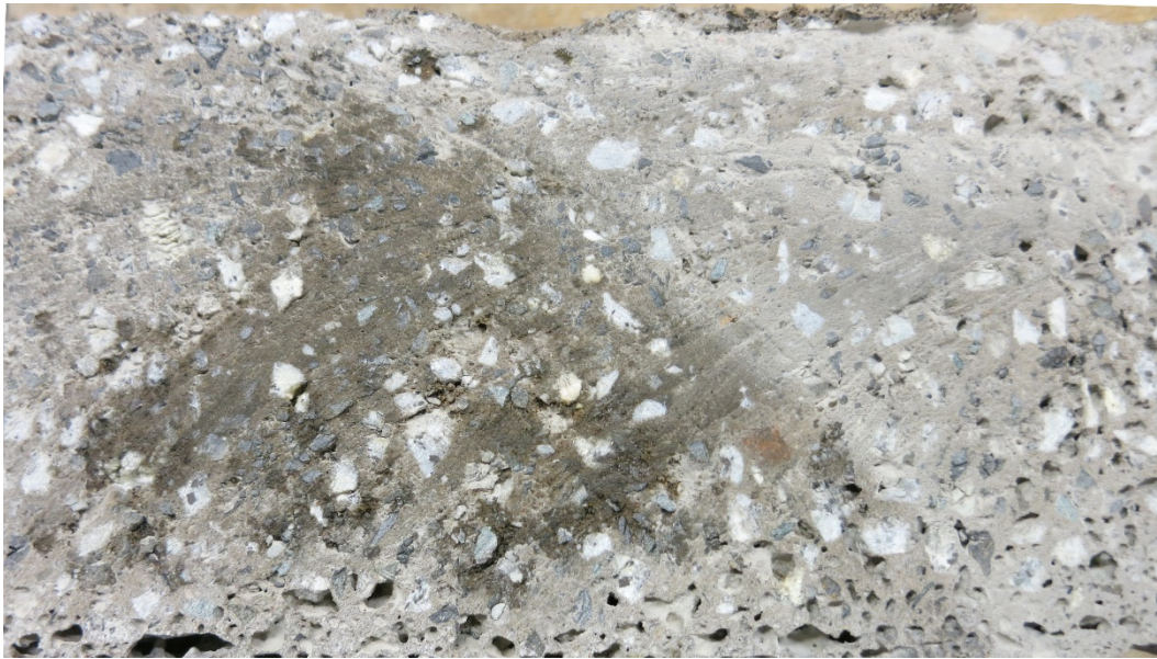
Figure 5.11 Cross section of 300x300x100 mm 3 specimen of Loy Yang brown coal fly ash geopolymer concrete.
