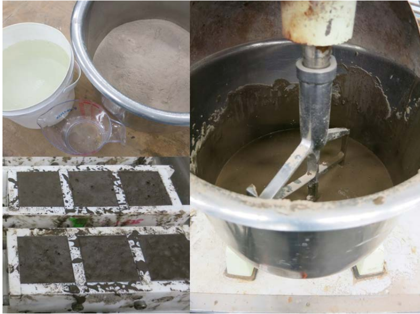
Figure 3.4 Brown coal fly ash geopolymer mortar: fly ash, sodium hydroxide and sodium silicate; mixing; and moulding.
