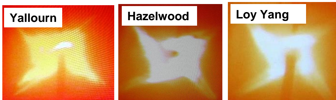
Figure 3.6 Flame pattern and intensity for the three air- dried Victorian brown coal samples under air-firing conditions of 1.2 MW
