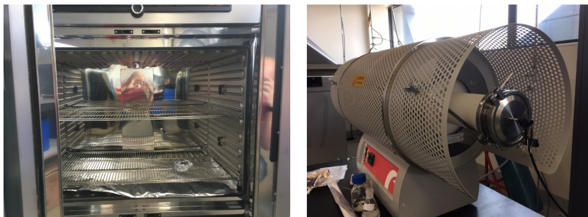
Figure 11 Picture of fan-forced oven and tube furnace
