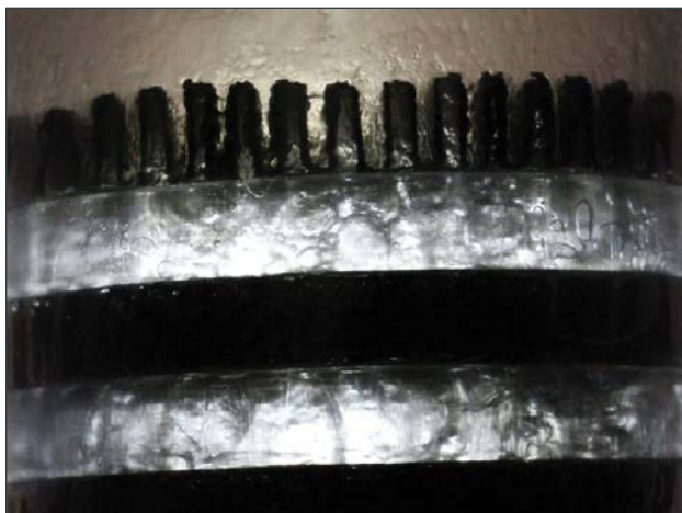
Figure 50: Internals of laboratory-scale WES froth absorber
