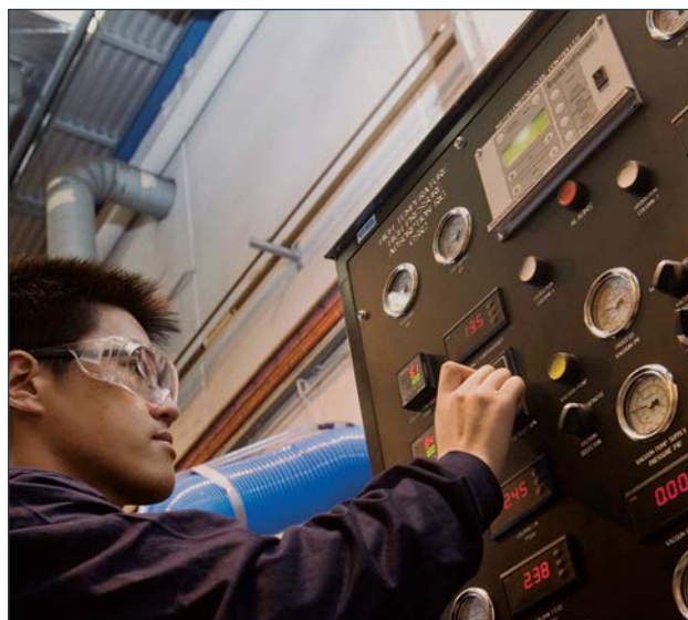
Figure 51: Operation of the pilot adsorption system on the HRL Mulgrave gasifier
