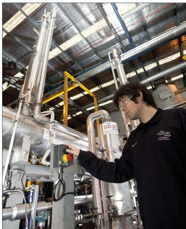
Figure 42: CO2CRC pre-combustion CO 2 capture rig at HRL Developments
