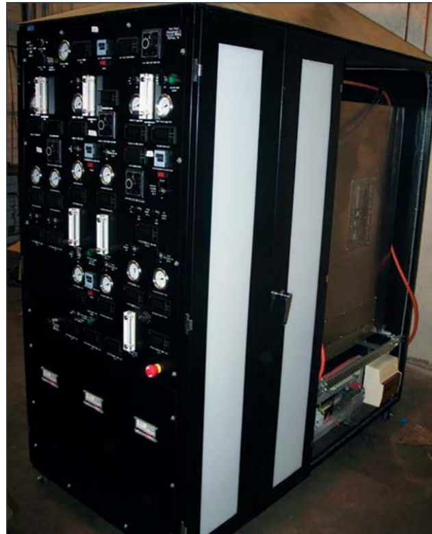
Figure 56: CO 2 CRC membrane pilot plant at HRL Mulgrave gasifier
