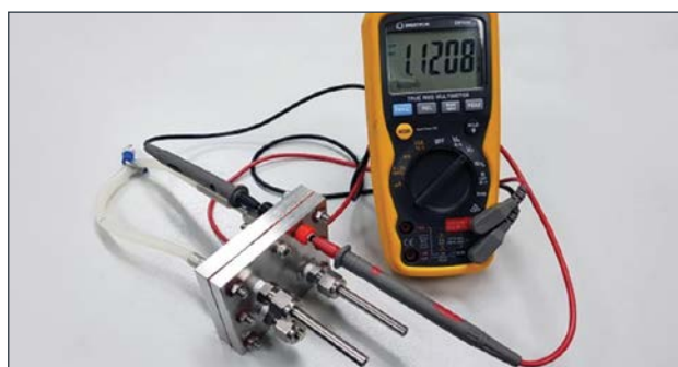
Figure 31: Prototype proton battery connected to a voltmeter
