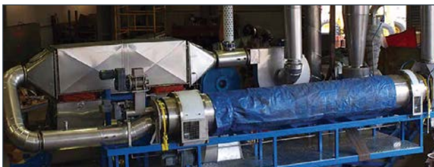
Figure 15: Pilot scale superheated steam rotary drum dryer system
