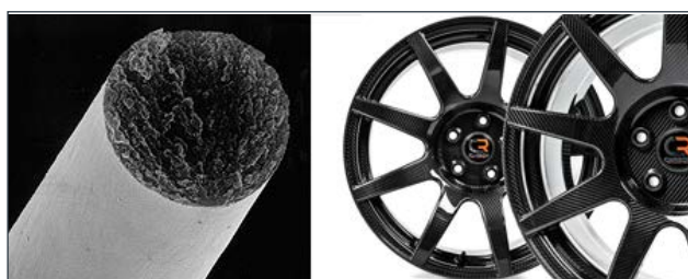
Figure 27: Individual carbon fibre and a carbon fibre car wheel made in Geelong
