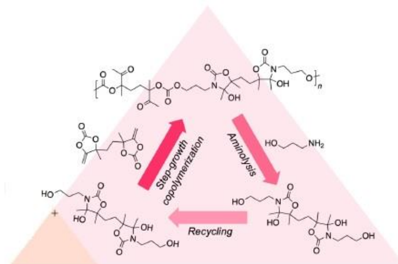
Figure 64: Example of a closed-loop polymerisation – depolymerisation system (Siragusa et al. 2022)
