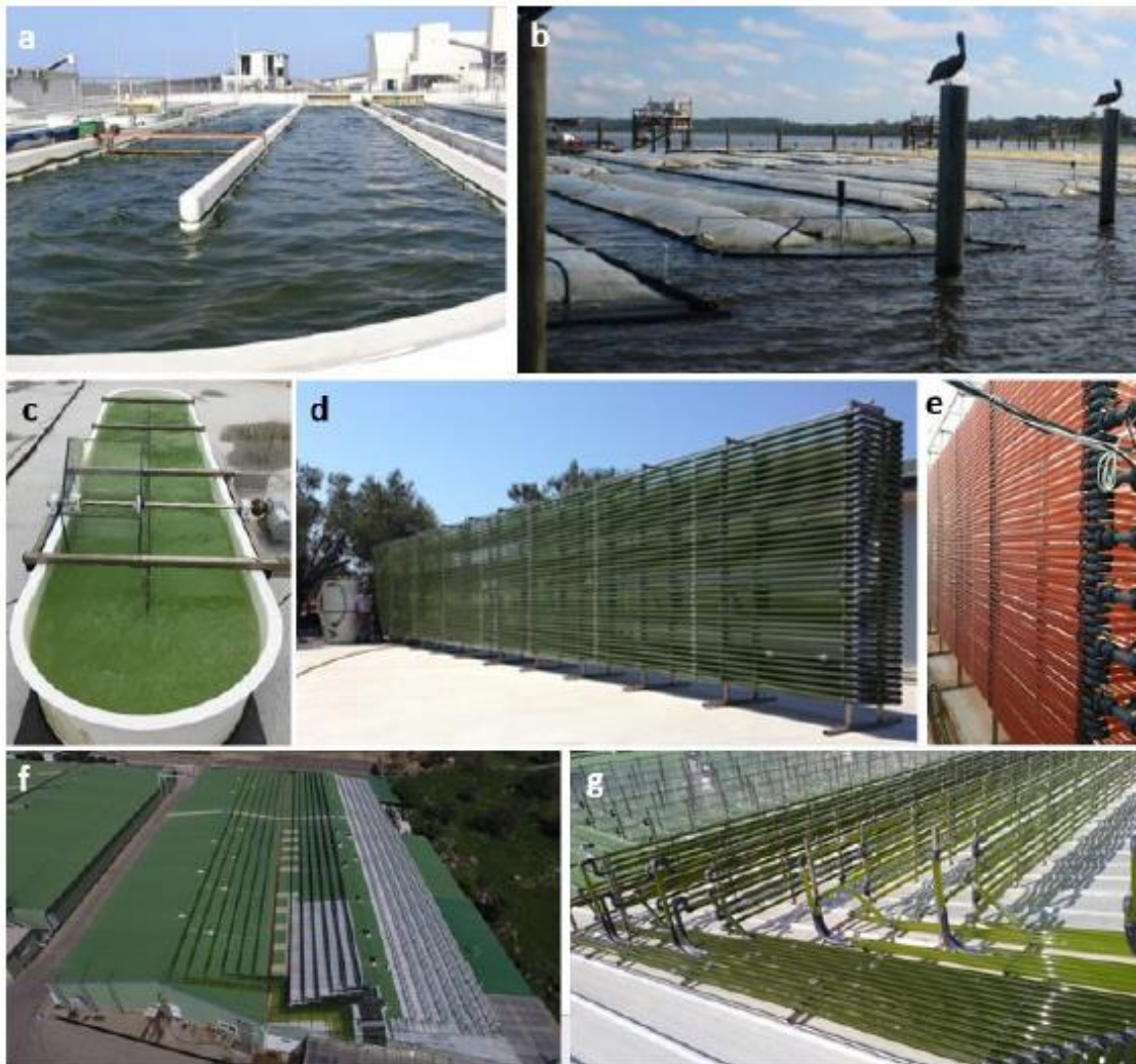
Figure 32: Examples of large-scale cultivation of photosynthetic microalgae and cyanobacteria. (a) Open pond (Israel) (photo credit Soren Nielsen) (b) Floating offshore closed PBRs with capacity 8000 L each at Algae Systems (USA) (c) 1000 L pond (Turkey) (d–g) Large-scale 40,000 L tubular PBRs at Akvatek (Turkey). 54
