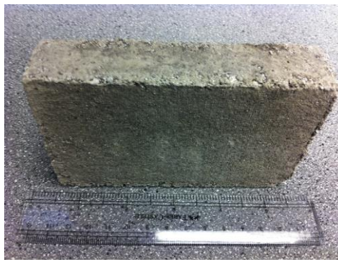
Figure 45: Slag-glass concrete block (Mahoutian & Shao 2016)
