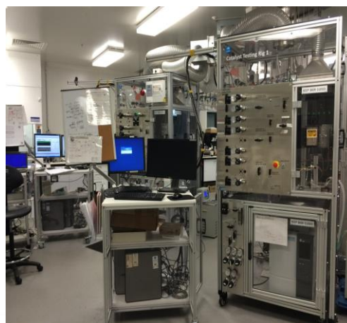
Figure 96: Multi-channel high throughput catalyst testing and lab scale catalyst testing rig at CSIRO
