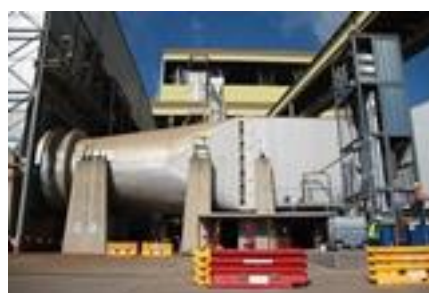
Captions (clockwise): 1. Monash University PhD-student, Mai Bui, records data from CSIRO's existing post-combustion carbon capture pilot plant located at the AGL Loy Yang brown coal power station in the Latrobe Valley, Victoria 2. & 3. (5656/5658): CSIRO's existing post-combustion carbon capture pilot plant scrubs CO 2 from flue gas at the AGL Loy Yang brown coal power station in the Latrobe Valley, Victoria 4. CSIRO and Monash University researchers working on CSIRO's existing post-combustion carbon capture pilot located at the AGL Loy Yang brown coal power station in the Latrobe Valley, Victoria
