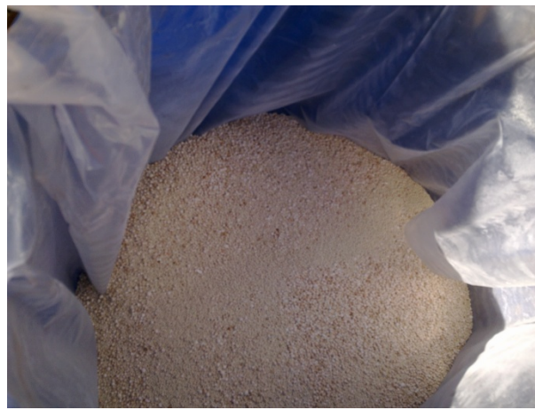
Figure 5.3.30 Mixed adsorbents due to fluidization
