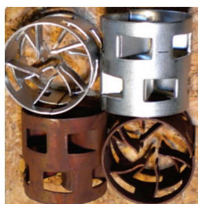
Figure 8. Photo of pall rings sampled from the absorber (top) and desorber (bottom) after the PCC campaign at Loy Yang
